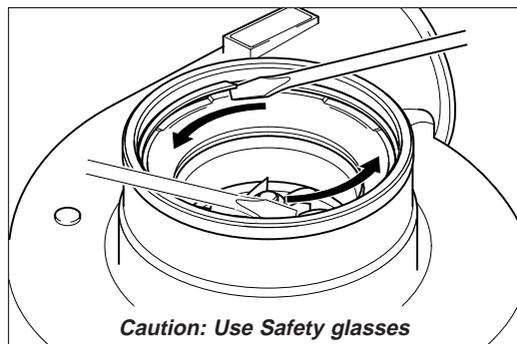
Push the screwdriver in an anti-clockwise direction to force the retaining ring out of the groove. Remove the retaining ring.
